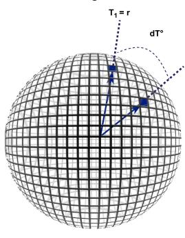
$$|T_1|*|T_2|*\cos(dT^\circ) = T_{1x}*T_{2x} + T_{1y}*T_{2y} + T_{1z}*T_{2z}$$
