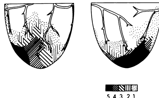
Figure 12. The area directly depolarized by a 20-V shock delivered during the TQ interval of normal sinus rhythm in five dogs. Different types of crosshatching represent the number of the dogs that had each area directly depolarized by the shock.
