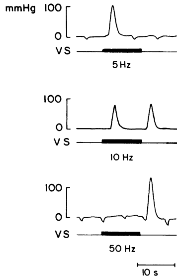
FIGURE 2 Influence of stimulation frequency on A and B contraction. Train duration, current intensity, and pulse duration were held constant at 10 s, 2.5 mA, and 1 ms, respectively. Note that the 5-Hz stimulus evoked only A-contraction whereas 50-Hz stimulus evoked only a B-contraction.
