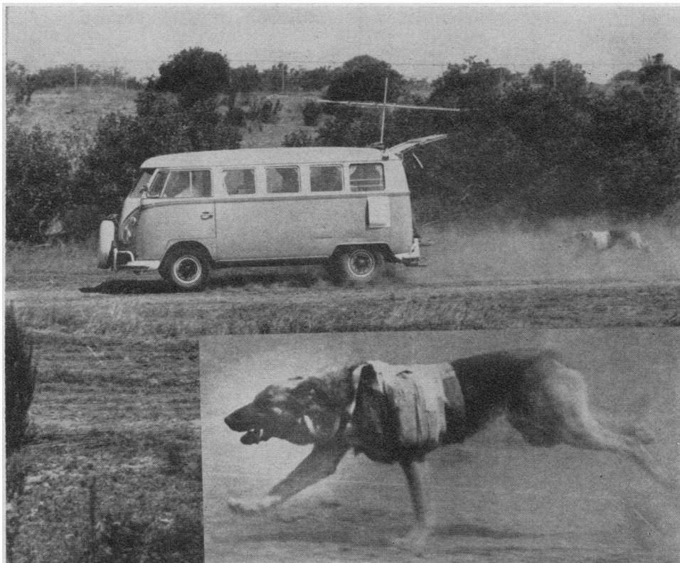
FIGURE 1 One of the instrumented dogs running at 22 miles/hr behind the mobile recording unit. The FM signal containing the flow-pressure data is telemetered from the instruments carried by the dog in saddlebags (insert) and received by the antenna on the bus, which in turn is coupled to the recording instruments.
