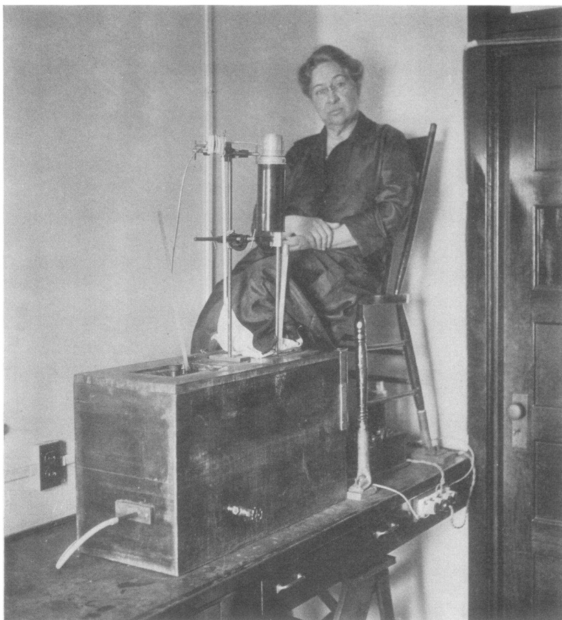
FIG. 1. APPARATUS USED IN MAKING CALORIMETRIC STUDIES ON THE EXTREMITIES
